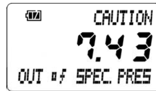
Caution display for Out-of-specification pressure (approx. -20 - +50°C)
